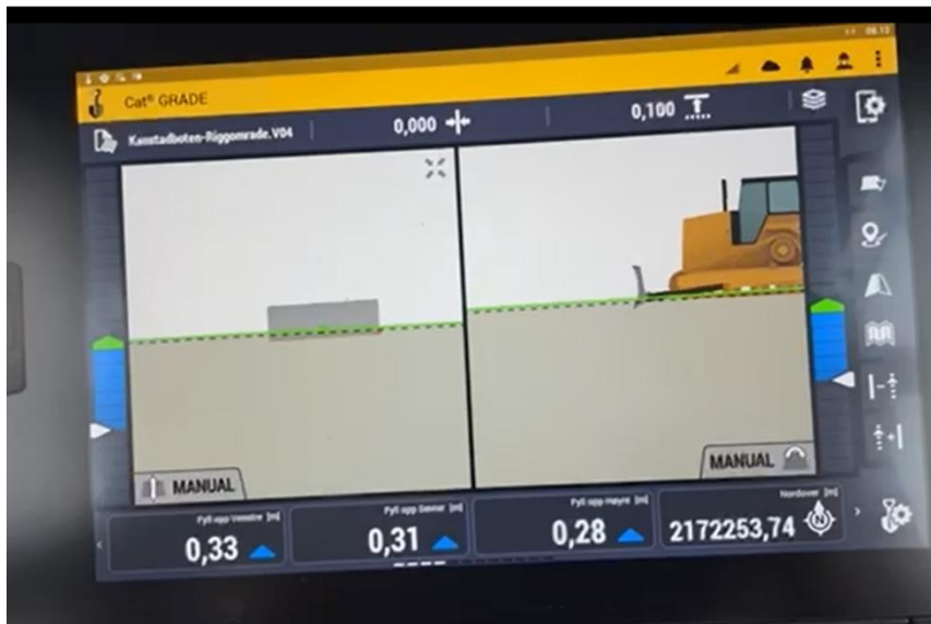
Figure 15: Example view of a bulldozer operator equipment. The left and right parts of the image show the front and side views. The numbers at the bottom indicate the altitude setting that should be used for the blade. During space weather activity these numbers fluctuate, even when the bulldozer is stationary, but if the activity is moderate there are no warnings in the display that the numbers cannot be trusted (Photo: Maskinstyring AS).
