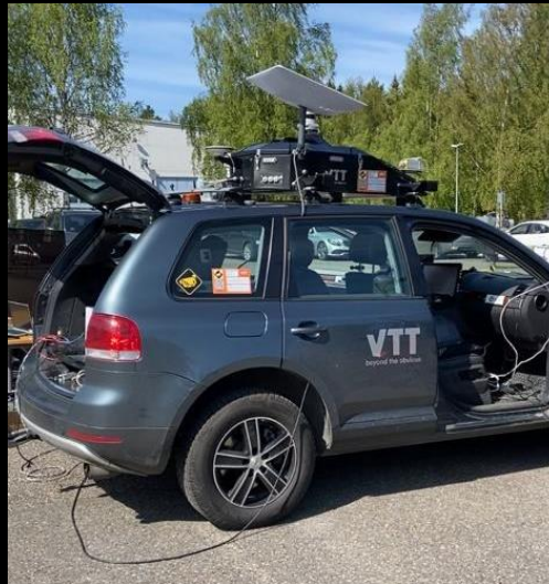
Starlink terminal on top of a car (Used terminal is designed for static/nomadic use.)
